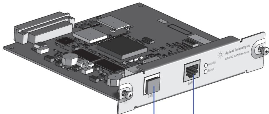
CAN port for “Hosted Module Support” connect to CAN port of the HPLC module that hosts this LAN interface card (if required). The CAN port of the “hosted module” connect with the provided CAN cable to a free CAN port on the LC system, see [page 52](#).
