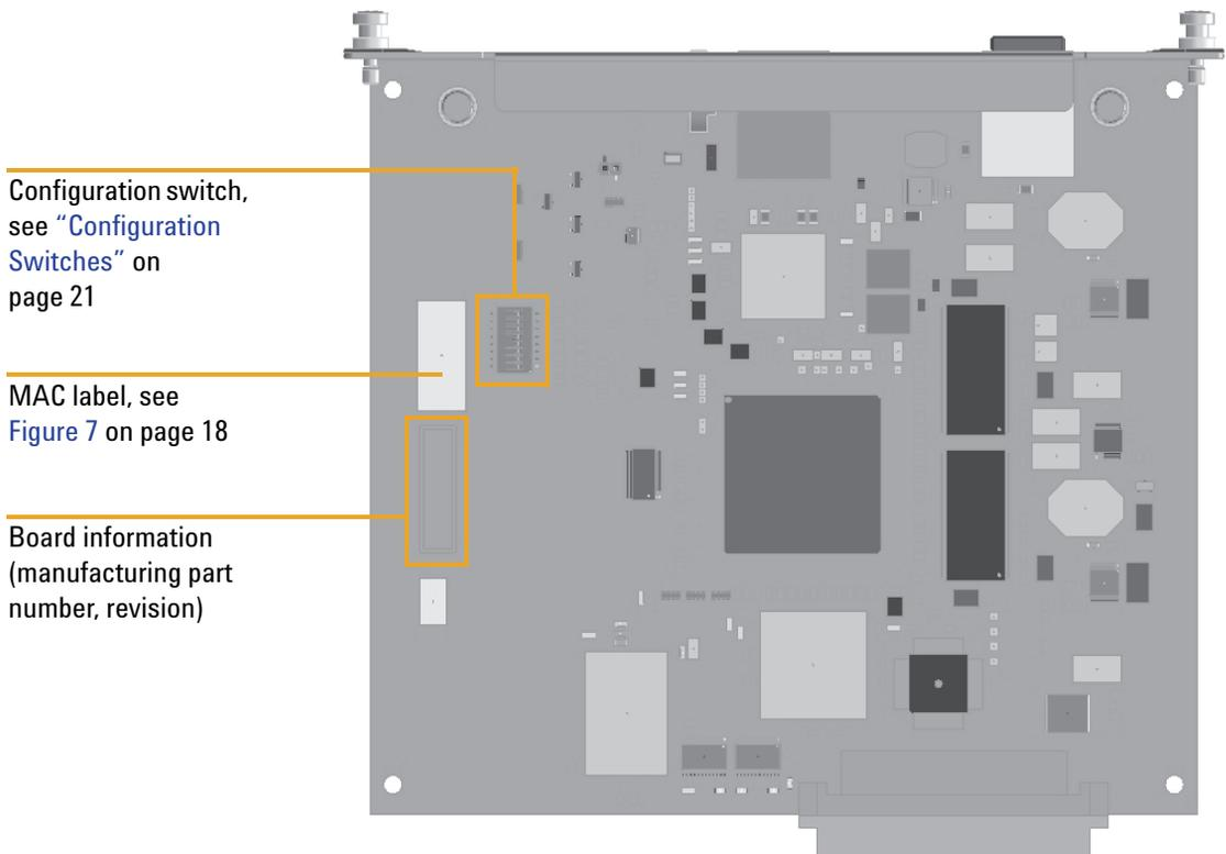
**Figure 6** Board Layout G1369C
