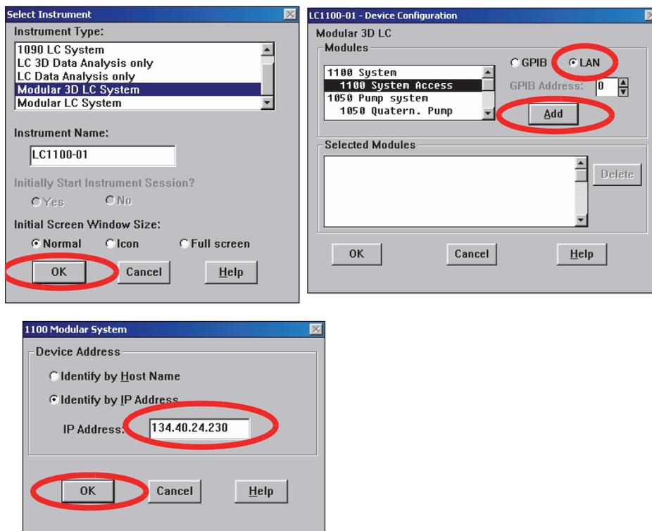
**Figure 41** Changing the TCP/IP settings of the Agilent ChemStation
