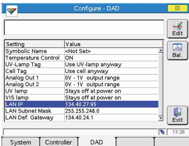
**Figure 30** Instant Pilot - LAN Configuration
