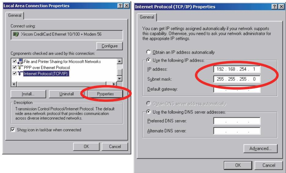
**Figure 40** Changing the TCP/IP settings of the PC
