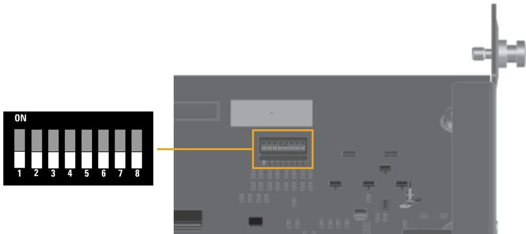
**Figure 10** Location of Configuration Switches
