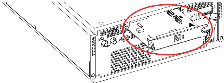
**Figure 8** Location of LAN Interface Card (e.g. 1100/1200 series detector)
