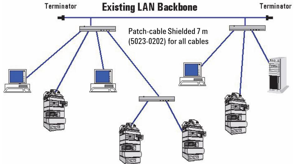
**Figure 4** LAN configuration with existing customer network
