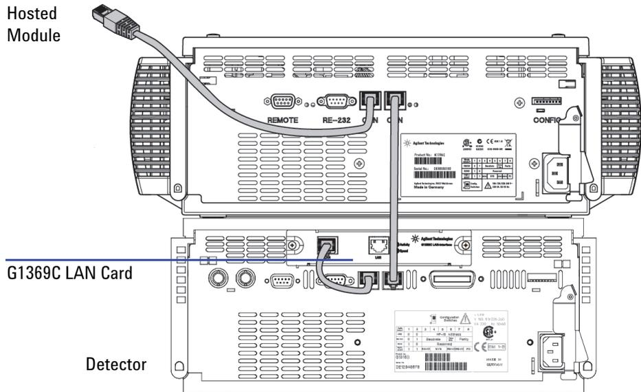
**Figure 43** How to connect hosted modules
