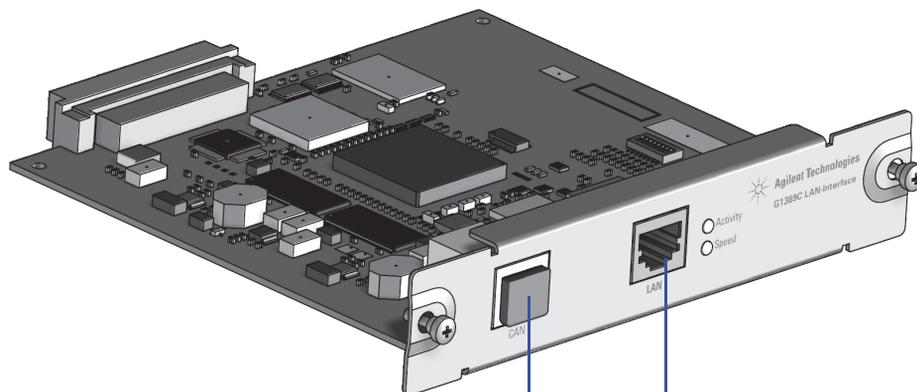
CAN port for "Hosted Module Support" connect to CAN port of the HPLC module that hosts this LAN interface card (if required). The CAN port of the "hosted module" connect with the provided CAN cable to a free CAN port on the LC system, see "[How to connect hosted modules](#)" on page 52.
