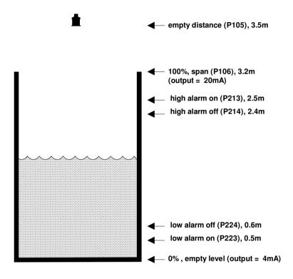
In this example, the blockbox and dB6 is being used to monitor a moving level within a vessel and is required to provide a 4 to 20mA output proportional to the level, over a range of 3.2m. In addition when the level rises to 2.5m, Relay '1' is required to give a high alarm and rest when the level falls to 2.4m. In the event that the level should fall to 0.5m then Relay '2' is to give a low alarm and reset once the level rise to 0.6m.
