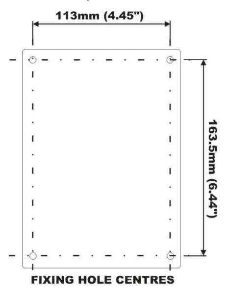
The full dimensions of the enclosure are as shown below.
