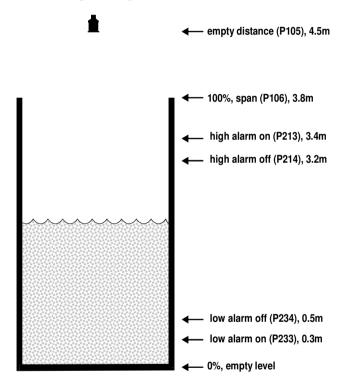
In this example, if the level rises to 3.4 m, then the high level alarm (relay 1) will come on until the level drops to 3.2 m. If the level falls to 0.3m, then the low level alarm (relay 2) will come on until the level rises to 0.5 m.
