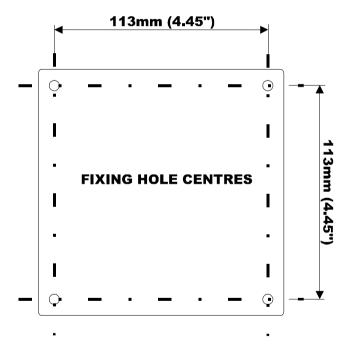
The blackbox should be mounted by drilling four holes suitable for size 8 screws (length and type to suit your application) And fix all four screws by removing the top cover to access the pre-moulded mounting holes which are located in the base of the enclosure under the lid retaining screws.
