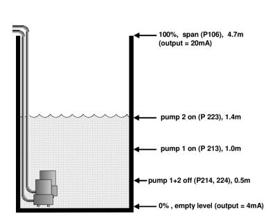
In this example a blockbox with dB6 is being used to control pumps on a **pump down** application, there are two pumps, and the **duty** pump is to be **alternated** between the pumps.
