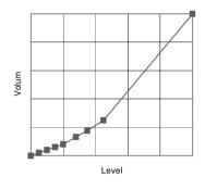
You should enter a level/volume breakpoint for each place where the vessel changes direction, and numerous where the section is slightly curved (mostly linear, but has got a small arc). You can enter any number of pairs between 2 and 32.
