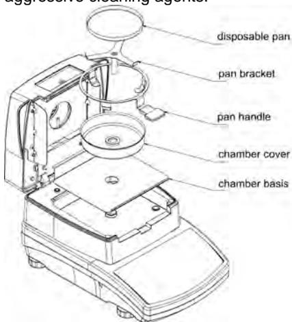
Do not use any abrasive agents or solvents to clean the moisture analyzer, as it may cause damage to the device and its components.
