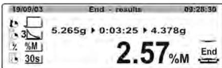
Additionally, the moisture analyzer automatically sends data, via the RS 232 communication port, printed in the **footer** (in accordance with pre-determined printout options – see group of parameters P6 Printouts).
