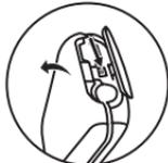
4. Press the battery toward the bottom of the phone and pull the battery out of the recess.
