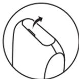
2. Between the phone jacks, there is a latch to aid you in opening the rear cover. Press the latch inward to release the rear cover.
