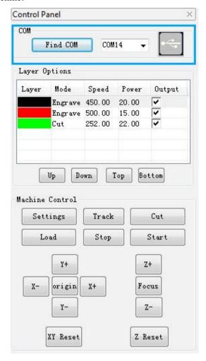
Click Find COM, if the machine is turned on and has been connected to computer through a USB cable, the correct COM will be showed and the USB icon will turn to Blue color.
