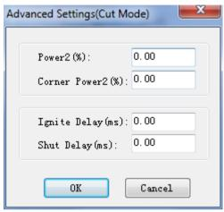
Power2(%):if your machine has two laser heads, you can set the power for the second head here.
