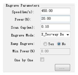
**Speed(mm/s):** max engraving speed of the laser while working
