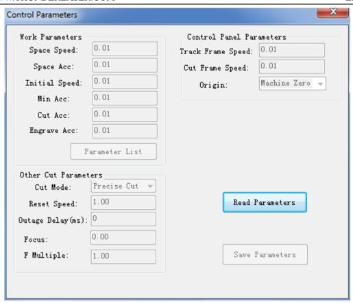
Click read parameters, the software will read the parameters saved in the main board as below:
