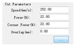
**Speed(mm/s):** max cutting speed of the laser while working
