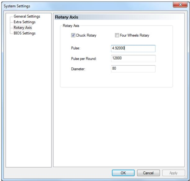
**Pulse:** this setting should be totally the same as the Y axis Pulse.
