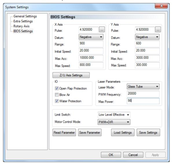
**Pulse:** send an pulse to control the machine. If this is not correctly set, the cutting size will be incorrect. If this happens, click to change the settings, after this setting, the software will find the correct pulse.
