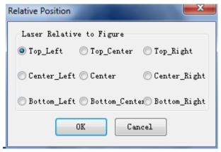
Choose the relative position to fit your work. The default relative position is the same as machine zero point. Look at the following examples to set relative position (the crossing point is the laser):
