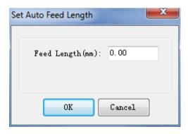
**Feed length:** the moving distance of U(auto feed Axis) axis between each process. This function is used only when the laser machine has a auto feeding conveyor.
