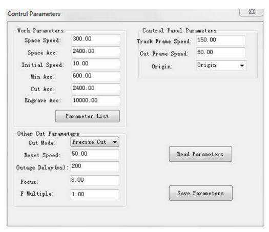
Select the parameters and change the settings and then click save parameters to save the data in mainboard.
