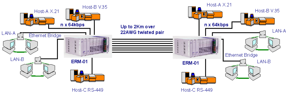
Figure 1-3 : Point-to-point Application of G703/64-RM
