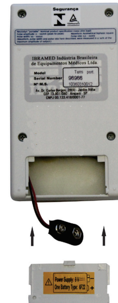
Figure 7. Type of battery used with device: IEC 6F22 - 9 Volts battery.
