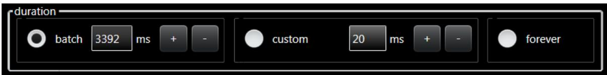
This group allows to choose which duration must be used when activating outputs (by pressing start button) and to modify these values :
