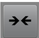
This button activates the platform batch J which has as standard configuration to move parts centered in long axis.
