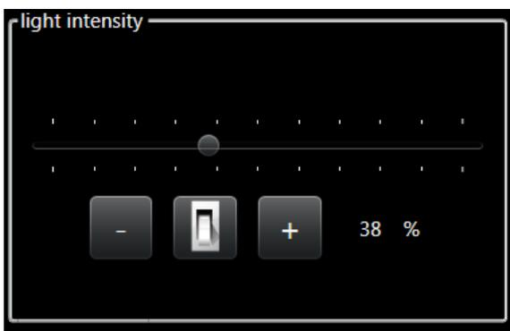
The light intensity group contains controls to adjust intensity of backlight.
