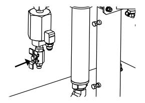
**12.** Make sure solvent regulator is dialed to zero. (Turn knob fully counter-clockwise)
