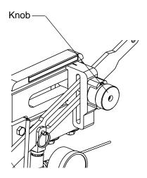
**2.** Turn main valve on the gun head to the recirculation position.
