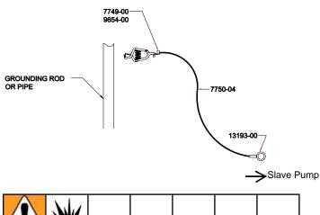
Whenever flammable or combustible liquids are transfered from one container to another, both containers shall be effectively bonded and grounded to dissipate static electricity.
