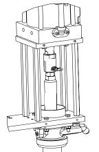
**4.** Material pump lube cup should be cleaned of old lube and refilled with new pump lube.
