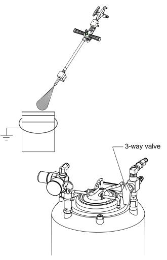
**3.** Exhaust air through the gun head until traces of solvent have been dissipated.
