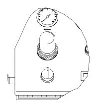
**4.** Switch machine recirculation to "ON".
