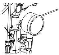
3. Open P/N 21192-00 on bottom of material pump.
