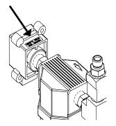
2. Open P/N 21228-00 on catalyst pump to recirculation position.
