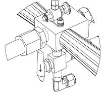
Make sure all the air is purged out of the catalyst pump on new start up.
