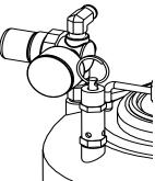
**13.** Carefully relieve any pressure in the solvent tank by slowly pulling the relief valve.
