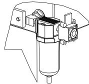
**8.** Slowly bleed the air pressure from the tank by lifting the ring on the relief valve.
