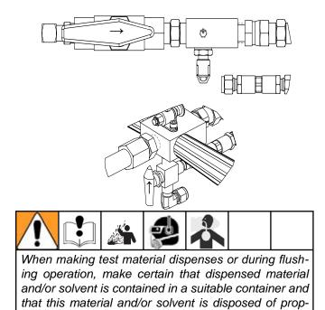
**7**. Flush gun head thoroughly. Turn 3-way valve on top of the solvent tank so the arrow is pointing up for air purge, for solvent turn the valve so the arrow is pointing down.
