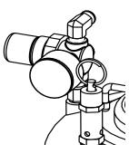
2. Place injection nozzle over a proper waste container. Turn 3-way valve on top of the solvent tank so the arrow is pointing up for air purge, for solvent turn the valve so the arrow is pointing down. Repeat air purge to blow solvent through the gun head.
