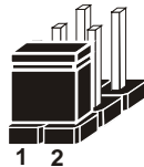
Jumper Block 1-2 pin close(enabled) Looks like this
