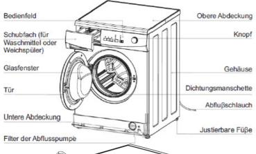
IMPORTANT: Unscrew the drain pump filter to let water run out when the machine is not used for a long time.
