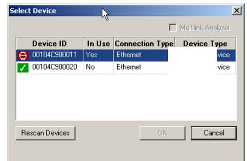
The software searches for all analyzers connected to the network and displays a list of available units in the Find Devices dialog. After you select a unit, the software assigns the IP address to the selected unit, completing the connection, then launches the software.
