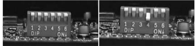
DIP Switch 4 in normal mode ("OFF", "up")
