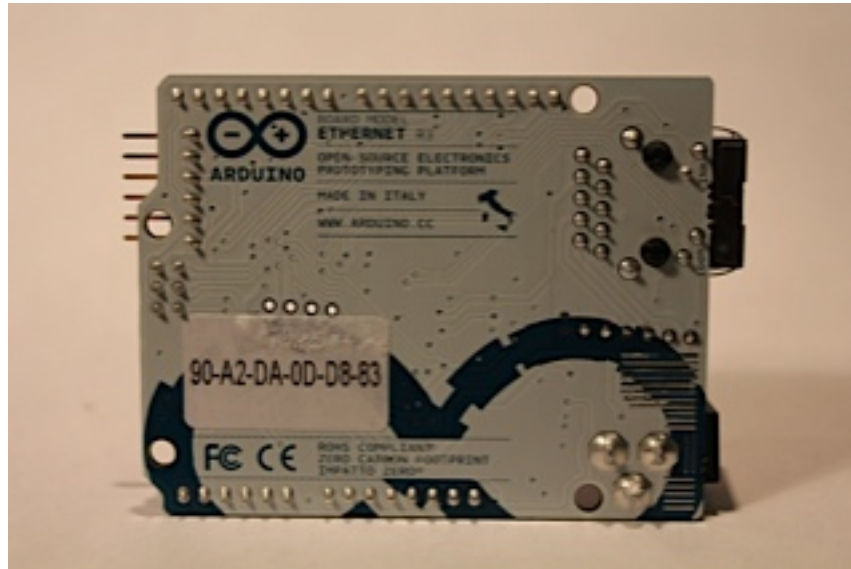
Figure 6: Finding the MAC address of your Ember board
