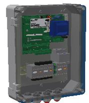
The exterior difference between the RLL610/611/660/661 Slave motor gearboxes and the RLL660/661/670/671 Master motor gearboxes are clearly visible on print circuit board X1 due to the connectors. At the Master version, all connection positions are provided with a connector. At the Slave versions, the connectors P3 and P7 are not mounted on the printed circuit board.
