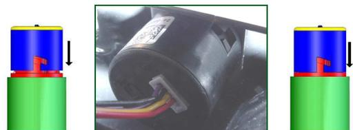
4. Turn the encoder till the mechanical stop;
