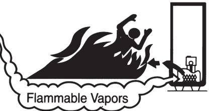
**⚠ Vapors from flammable liquids may explode and catch fire causing death or severe burns.**
