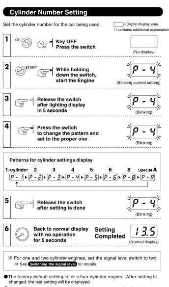
If the engine is a two cycle engine, multiply the number of cylinder by two. (e.g., For a two-cycle three-cylinder engine the setting would be six.)
