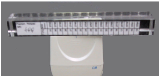
Figure 6.3 Positioning the phantom on the probe for SQV
