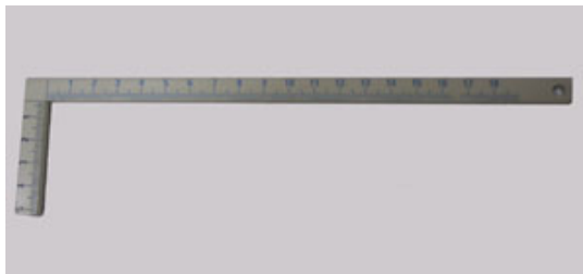
Figure 15.1 L-gauge for measuring the phalanx
