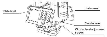
4 If the bubble is not centered, shift the bubble to the center of the circular level by rotating the three circular level adjustment screws on the circular level with the adjustment pin included in the package.
