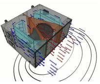
transmission line paths as well. Its working principle is an hybrid combination between a short transmission line and an overdamped reflex load. Moreover, the maximization of the mutual coupling between the drivers increase the fastness of the transient response while maximizing the overall energy efficiency as well.
