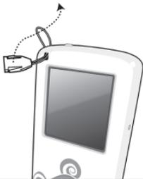
Insert the Strap connector through the rope's loop until snug.
