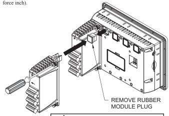
WARNING: Disconnect all power to the unit before installing or removing modules.
