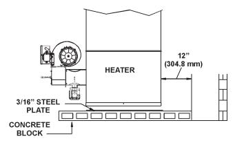
PROPER INSTALLATION ON COMBUSTIBLE FLOORING FIGURE 2.
