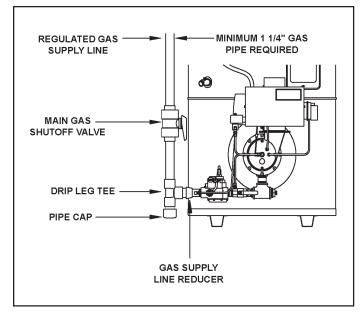
GAS PIPING AND DIRT LEG INSTALLATION FIGURE 9.
