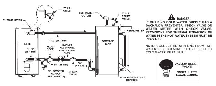
NOTE: WHEN USING A State T-140, 200, 350 OR 400 STORAGE TANK, USE LOWER 3/4" OPENING FOR TANK TEMP. CONTROL
