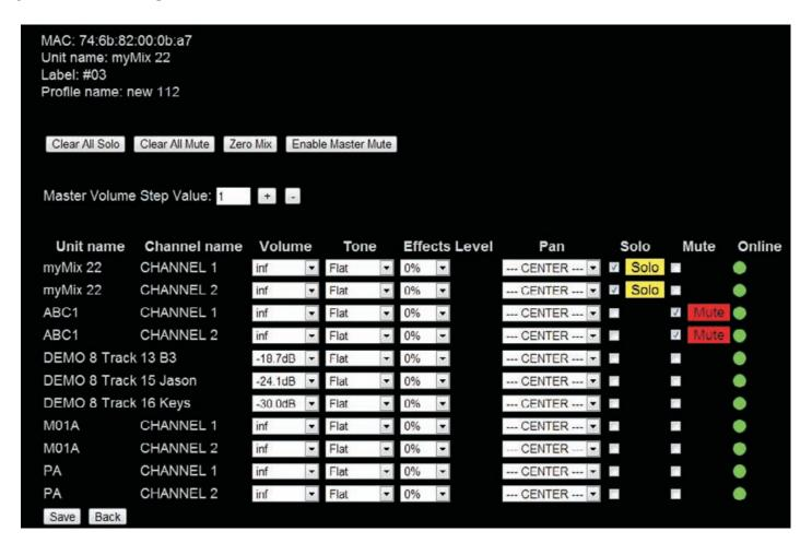
Edit Mix - Page is showing the current mix parameters of the myMix device at opening of the page. Note that changes made manually on the myMix itself after the page is loaded are not reflected in this display. That's why we recommend not to leave this page open too long (unless there is nobody operating the myMix manually).
