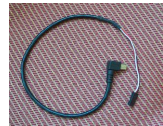
Custom cable with mini USB to male RC servo connector
