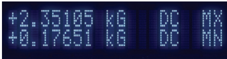
The display configured to show both the Maximum and Minimum DC field values
