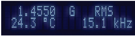
The display configured to show the RMS field value and frequency, and the probe temperature
