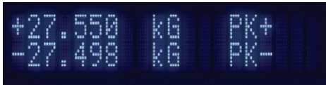
The display configured to simultaneously show the positive and negative Peak readings
