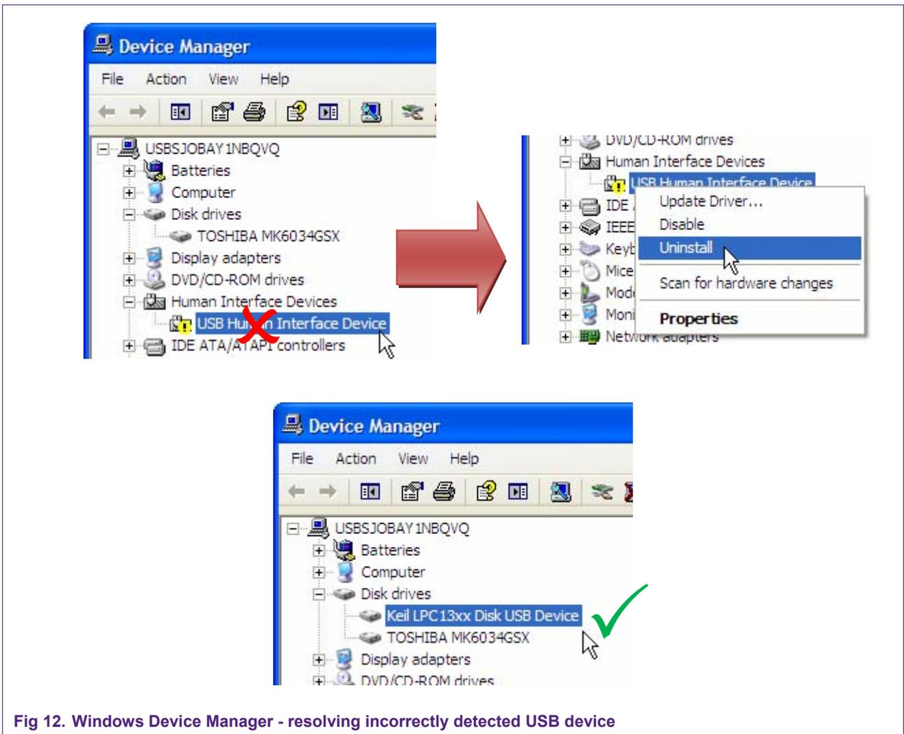
Fig 12. Windows Device Manager - resolving incorrectly detected USB device
