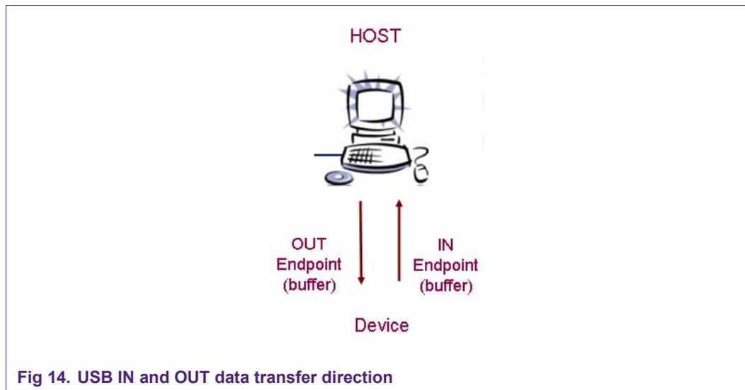
Fig 14. USB IN and OUT data transfer direction
