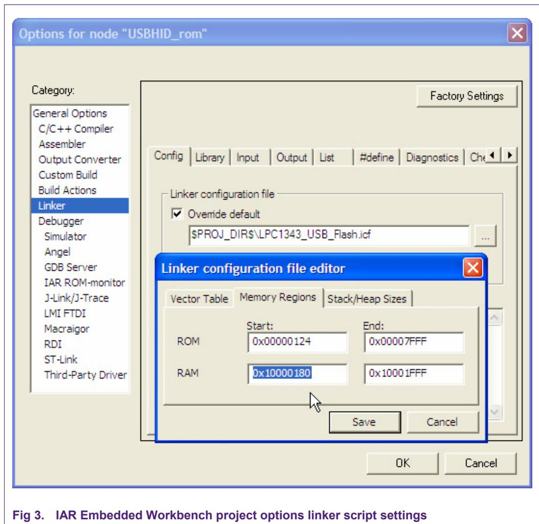
Fig 3. IAR Embedded Workbench project options linker script settings
