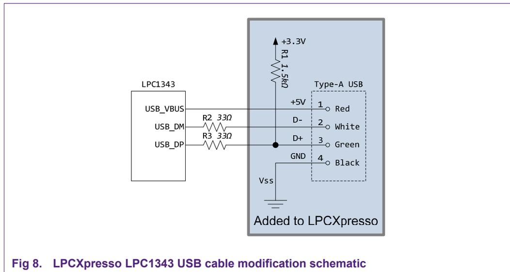
Note: Rather than building a cable or wiring a USB Type-A connector, you could take an existing A-B USB cable and cut the B connector off of it. Then the A side of the cable could be stripped and soldered onto the LPCXpresso board.
