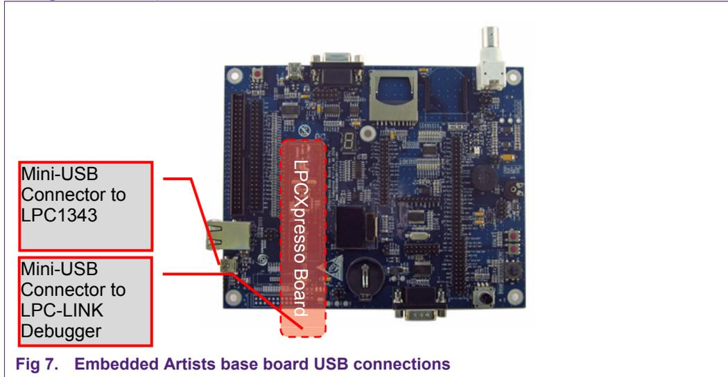
Fig 7. Embedded Artists base board USB connections
