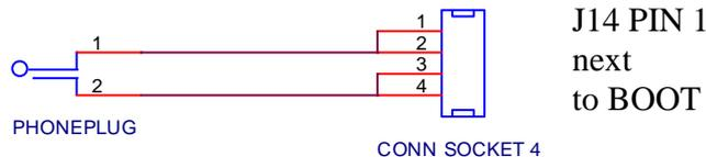
This plug is inserted into the 1/8" socket next to the RJ45 MIC socket on the back of the IC706.
