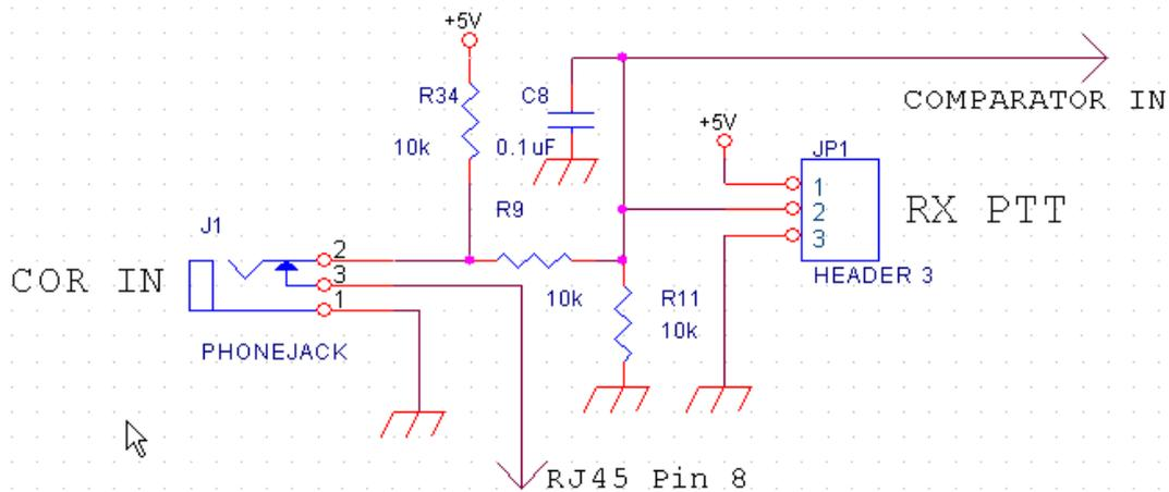
With nothing connected the COR input sits at about 3.3v so when using a open collector input set the threshold to about 2v for good operation. If the open collector device ins turned on when a signal is received leave the “Open Squelch Above Threshold” box unchecked.
