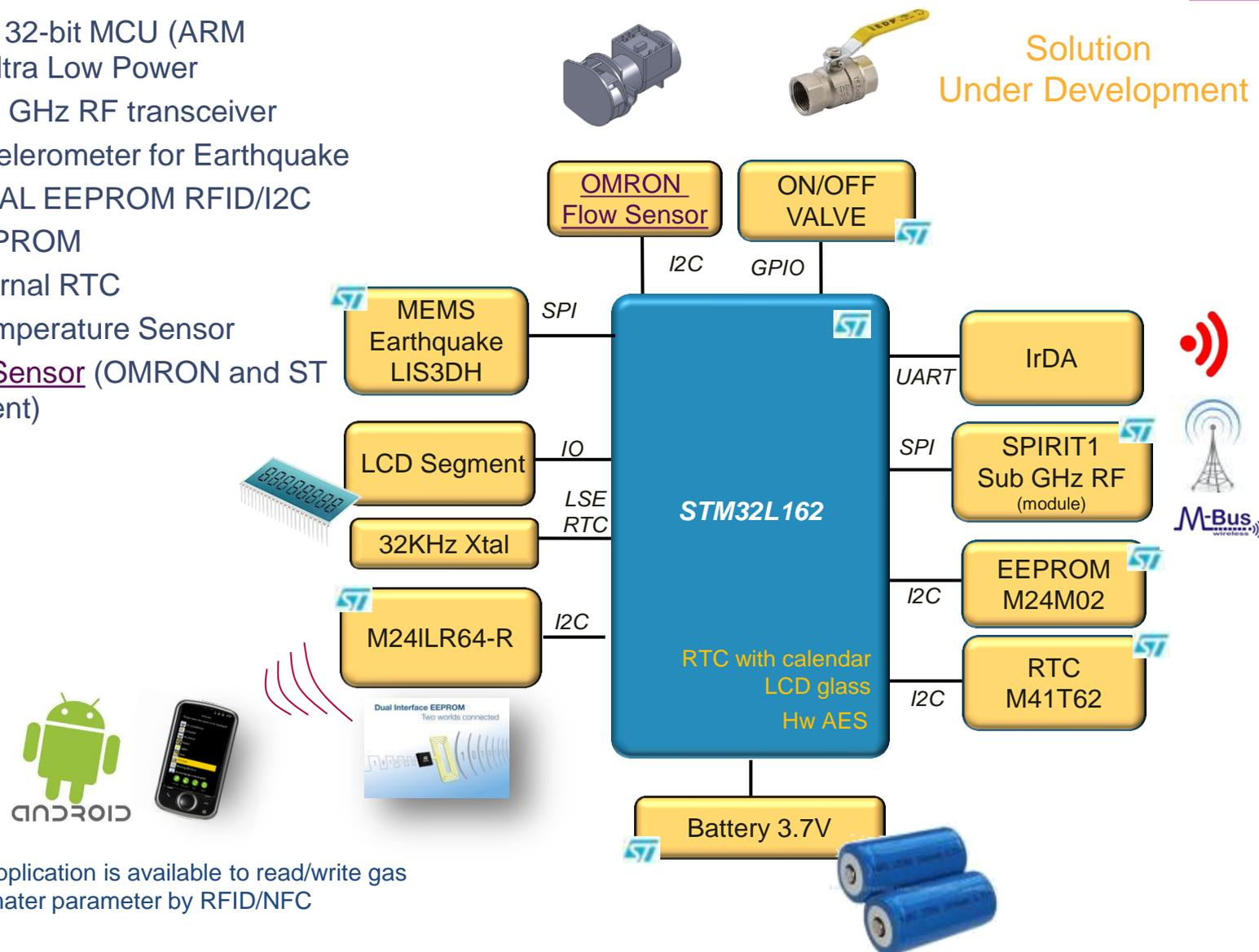
Android Application is available to read/write gas meter parameter by RFID/NFC
