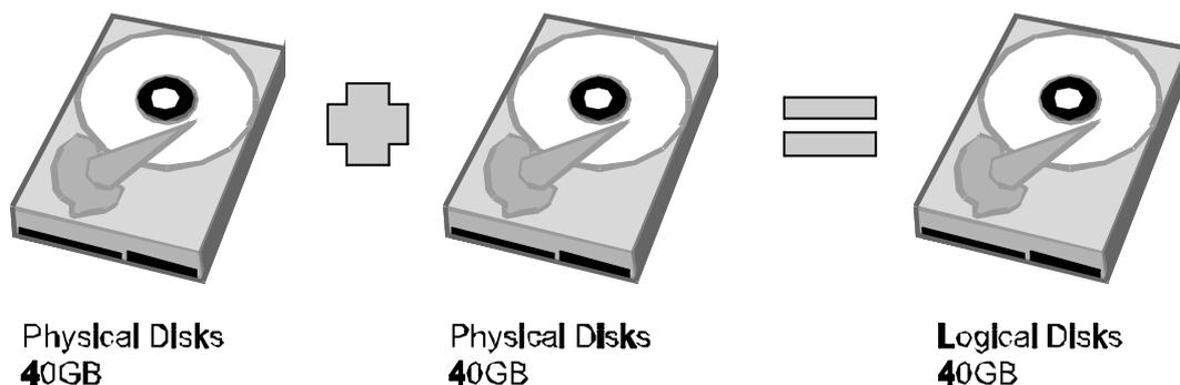
Mirroring offers the highest level of data protection. If one disk in the array fails, a backup is always available. Mirroring is typically used in mission-critical systems, such as payroll, accounting, and ERP databases.
