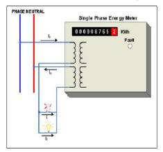
Fig:-2 Normal P & N connection
