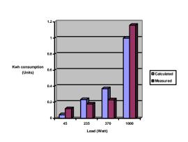
Bar chart of Kwh consumption at various Inductive load
