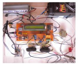
Fig:-5 Designed energy meter
