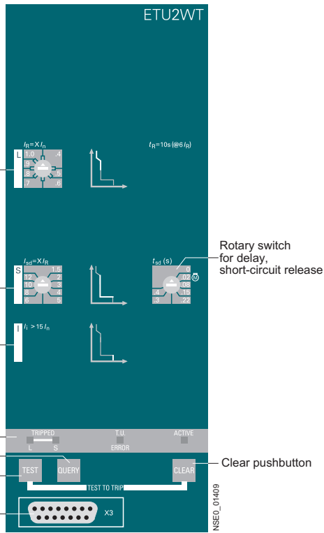
Electronic trip unit version ETU2WT "LSI"
