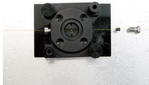
Flow Cell (Close-Up)
