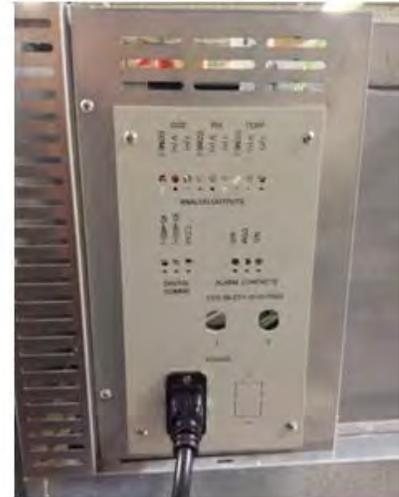
Analog outputs as either milliamps (4-20mA) or voltage (0-5V) signal output that represents each of the displayed temperature (and humidity) values. These options can be used for connection to in-house data acquisition, recorder, or alarm system.
