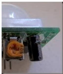
Least sensitive: Need significant movement for sensor to trigger. Detects movement from about 4 steps away.
