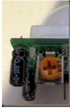
When you move the 104 labelled potentiometer all the way to the right (min position), the LED will remain on for 1 second after movement is detected. When the LED turns off, it will remain off for 3 seconds before the sensor will trigger again from any further movement.
