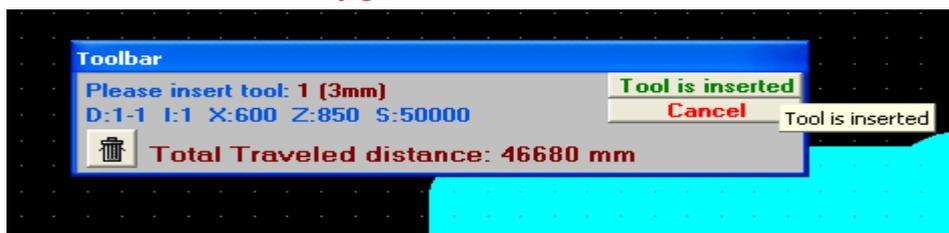
18. Now the board routing will start and you can see the circuit tracks being made by the machine, if anything is not going right, for example the routing depth is not right or machine offset is not properly set, you can press the **ESC** key to stop the machine.
