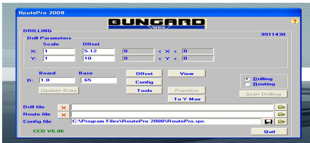
3. First load the **Route File** by clicking on the browse bottom icon shown below. From the browser button navigate to **.plt file** that you have previously created while saving the milling data in **ISOCAM**.
