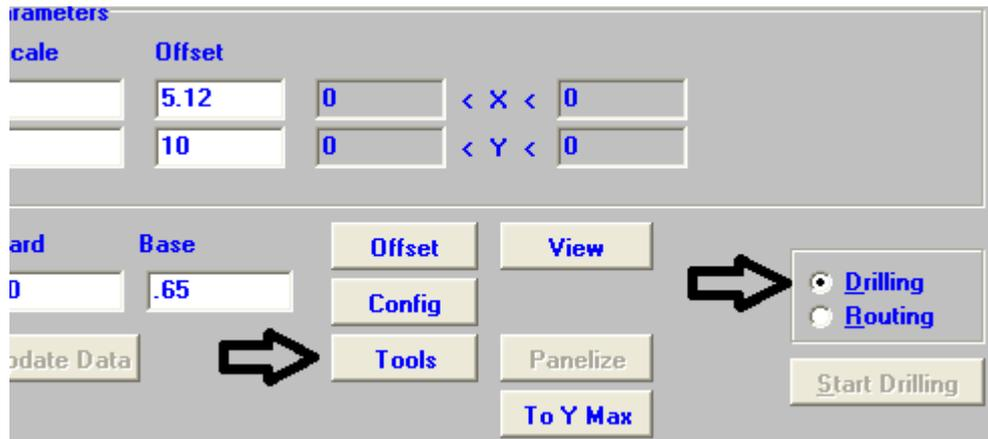
21. Now in the Drill tool options, enter the drill depth **2** under the **+mm** column for all the rows including T1, T2 ..... Tx, press **Update** and then **OK**
