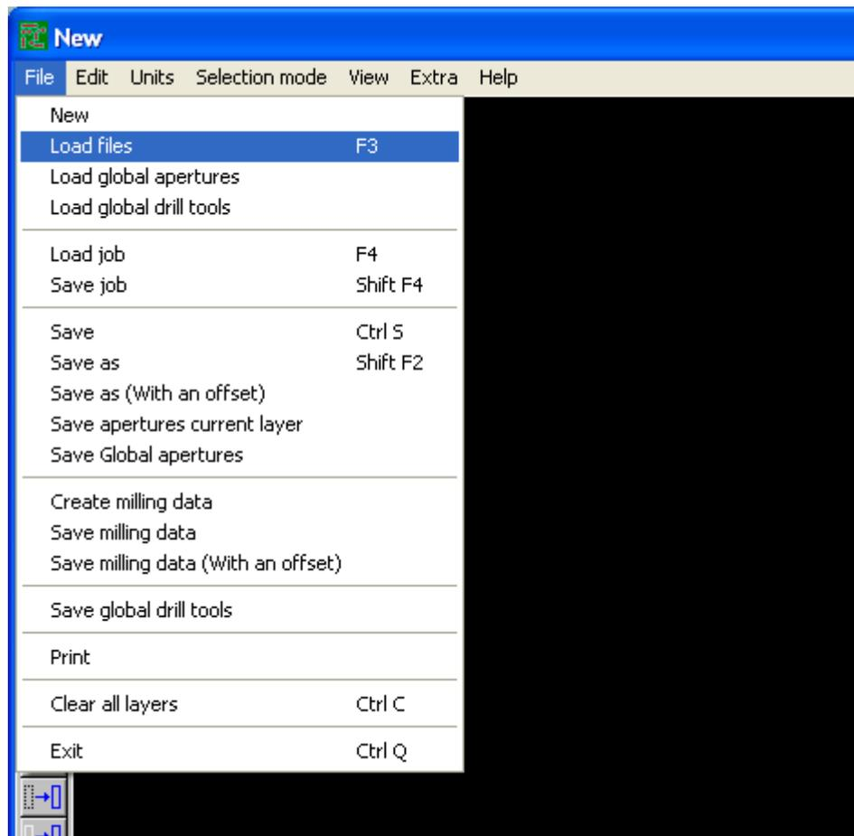
3. Now navigate to the folder where all the Gerber/CADCAM PCB design files are located. Only select Bottom Copper and Drill files.
