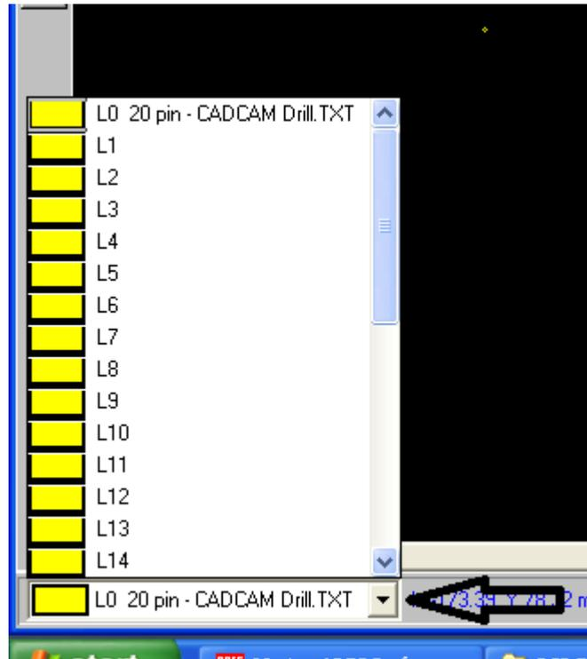
19. After selecting the Drill file you will observe the file name with full path on the top of ISOCAM window e.g C:\Documents and Setting\.....\20 pin – CADCAM Drill.TXT
