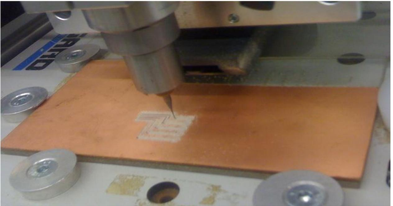
The machine is operating in routing mode.
