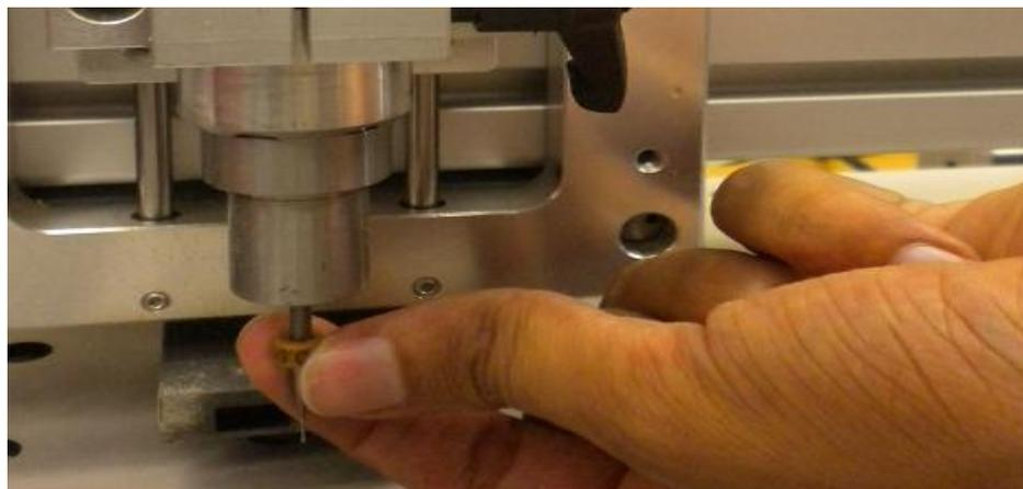
7. When the Collette is loosen enough and the bit can easily slide in, insert the bit upto its brown collar and tighten the collete for which you now need to rotate the **bit lock** clockwise as shown in the figure below
