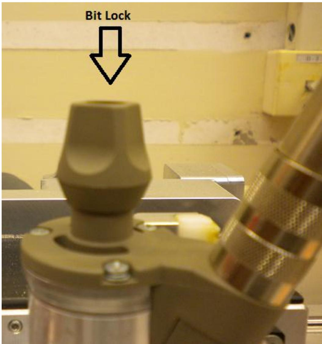
6. First you need to loose the Collette so that you can insert the bit, to do that, push the **bit lock** downwards gently and rotate it counter clockwise, with two or three rotations the Collette will be loosen, to check whether the **collate** has loosen, try inserting the bit in the Collette gently if you unable to do so then try repeat the above steps again until the Collette is loose.
