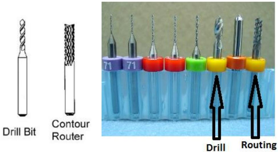
4. In physics lab you can locate the routing bits in a box labeled "PCB Machine" located by the side of CCD2 PCB Machine. Only 0.6 mm routing bits are available with brown colored collar as shown below
