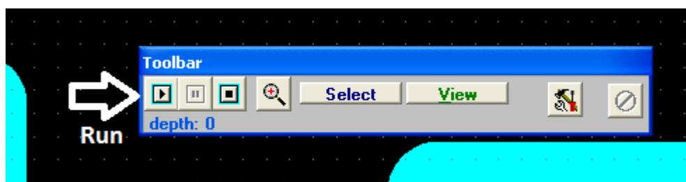
24. Now the machine will drill holes through the circuit board, remember if the holes haven't been drilled thoroughly through the circuit board, then increase the drilling depth under the **+mm** column shown in the previous step.
