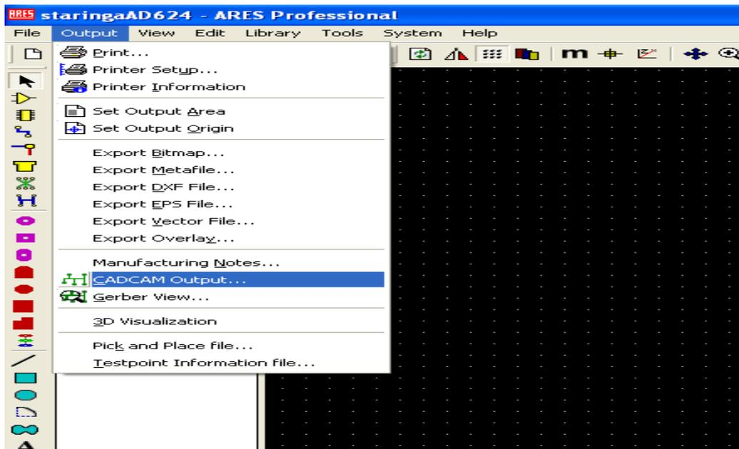
7. From CAD/CAM output window make sure that **Mirror** and **RS274X** is selected. Now specify the output folder where you want to save the Output GERBER/CAD/CAM files. Please note that on the left it shows all the layer that it will export: Top Copper, Bottom Copper etc. files. You only need to check Bottom Layer and Drill boxes, rest are of no use here.
