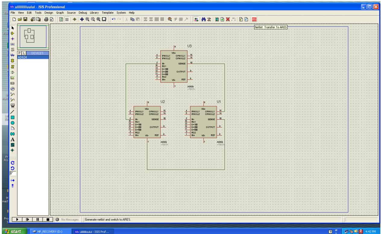
3. Once finished with the design click on the red button shown in the figure below. It will generate the Netlist of components and open the ARES interface.
