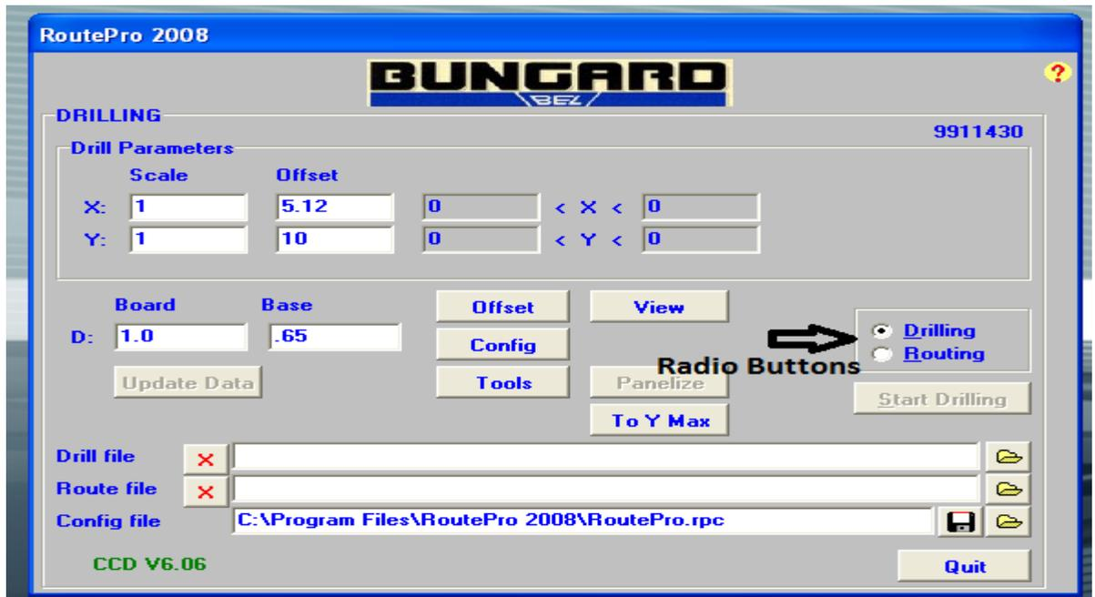
6. **Offset** defines the point on PCB from where you want this machine to start its work. By setting the **Offset**, you set the origin of the machine. Let's configure the machine offsets for drilling operation.
