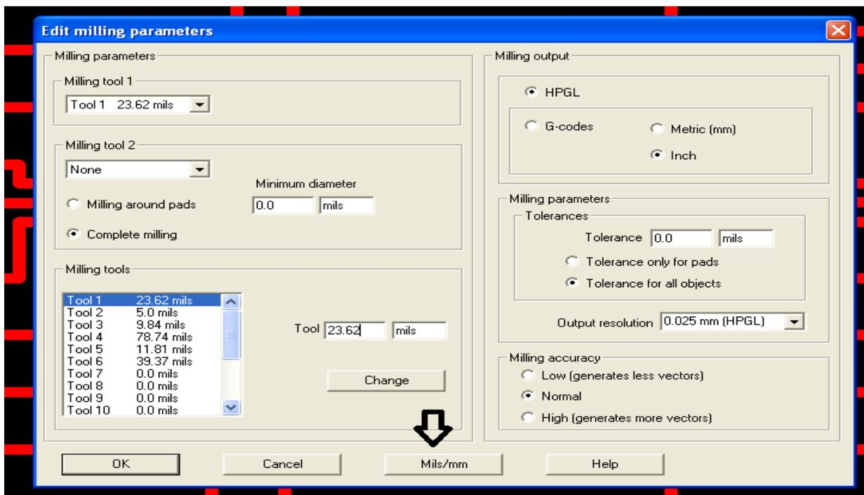
11. Now enter **0.6** in the **Tool** option and then click on **Change** and then finally click **OK** as shown below. Also make sure that the Milling output should be on “**Inch**” option.
