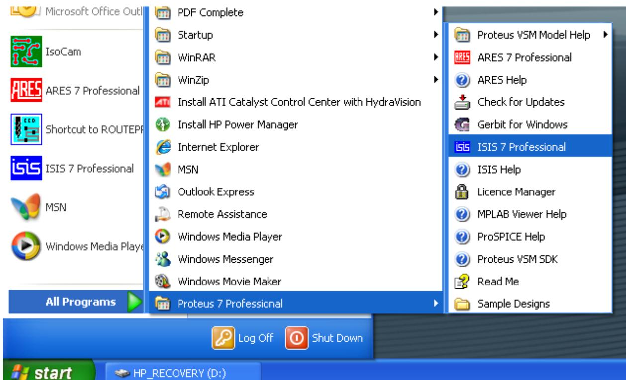
2. After opening Proteus you can make any circuit design using Proteus available components. Make sure that the components you use must have their PCB footprint available in the package (or in other words, they must have the component packages for ARES). For further detail use Proteus Help menu.
