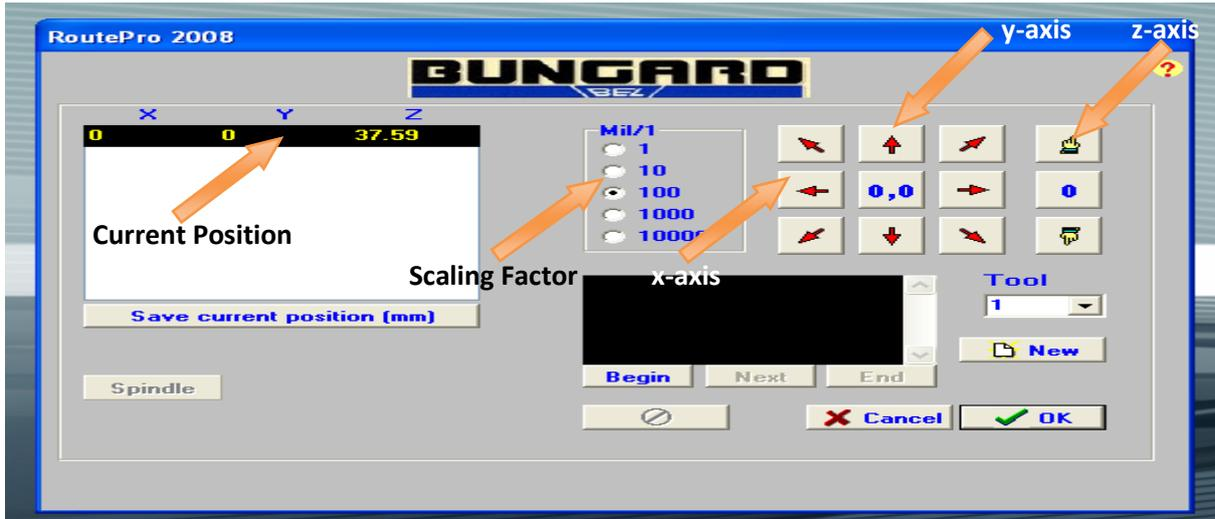
9. By clicking on the “**red arrows**” you can adjust the machines initial position of operation. Adjusting the machine’s initial position by putting the offset means that the machine will start making the circuit from that point. Once you are satisfied with the initial position (Offset points) click **OK**.
