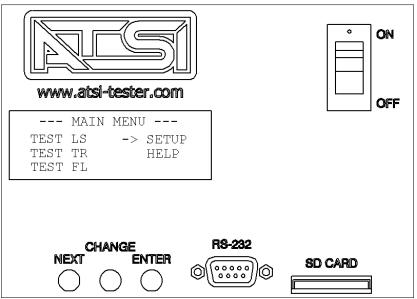
Figure 3. Operator Interface
