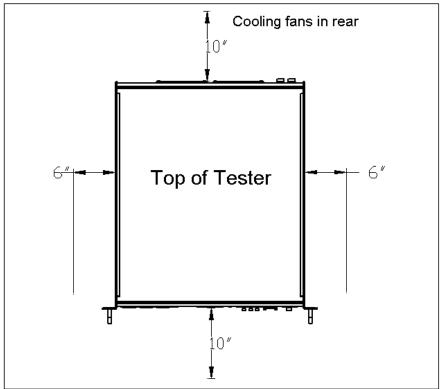
Figure 2. Minimum clearance distances.
