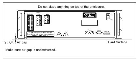
Figure 1. Tester placement.
