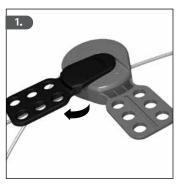
Rotate the black locking lever to the left to place the hasp in the fully open position. This will set the internal locking mechanism to the maximum opening diameter to accommodate the cable.
