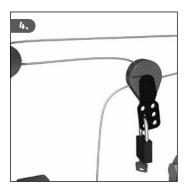
Placement of the lock shackle into any one of the six holes will prevent the locking lever from being opened.
