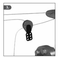
Rotate the black locking lever back to the right and into the locked position. Pull the cable to the desired length. The cable cannot be removed from the locking device once the black lever is in this position.
