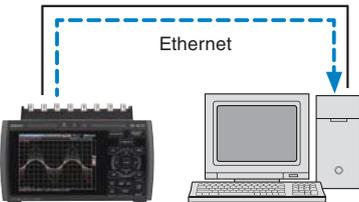
Set an IP address on the logger, connect the logger to a PC through a LAN and have the FTP client software copy the data.
