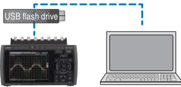
Plug a USB flash drive into the logger, copy data on the drive. Then, pull out the drive from the logger and plug it into a PC.
