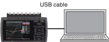
Connect the logger to a PC, have the PC recognize it as an external drive and copy data.
