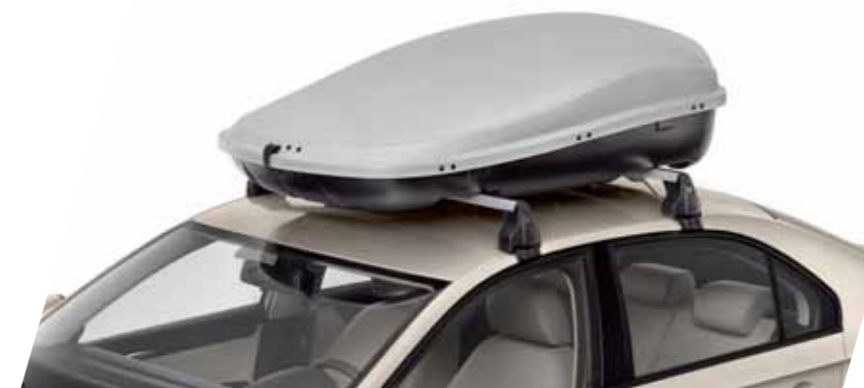
450L LUGGAGE TRUNK. Double plastic weather resistant walls. Weight: 18 kg. Maximum load: 50 kg. Used together with roof bars. 000071180A
