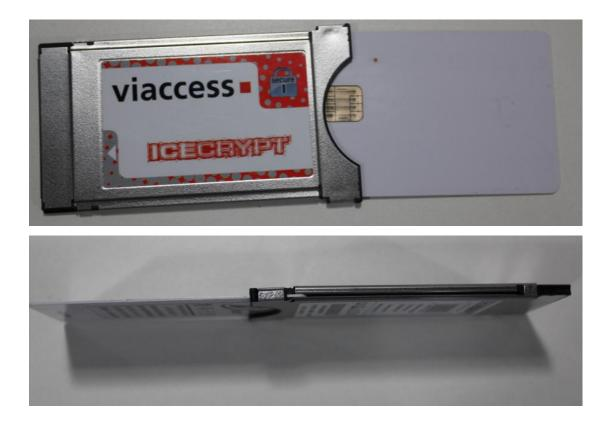
Step2: Insert the CAM into the TV Box CI slot. The thicker side(normally the side with brand and model information) of the CAM should face the up side of the box. The CAM should be inserted with the correct side up otherwise it won't be recognized by the box.
