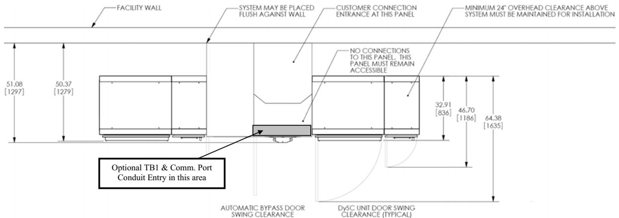
Figure 2 - Typical System Layout, Front View (800A ER model shown)
