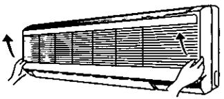
Hold the panel openers at both sides and pull up the front panel.
