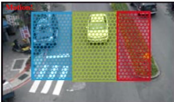
**The moving object will be detected when it is in any of the 3 motion areas, and the motion is triggered!**
