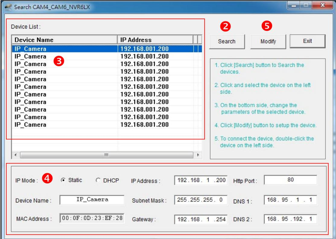
The screenshot shows the 'Search CAM4\_CAM6\_NVR6LX' application window. It features a 'Device List' table, a 'Search' button, and a configuration panel for the selected device. A red box highlights the device list, and another red box highlights the configuration panel. A third red box highlights the desktop icon for the software.
