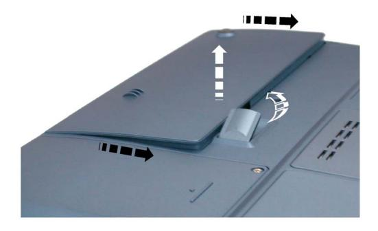
3. Hold the battery at the finger grip and lift it out of the compartment.
