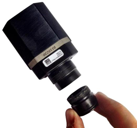
Be careful when you replace the infrared lens. The lens has a delicate anti-reflective coating.
