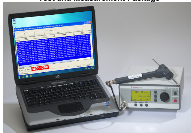
R-506, TV-2 Dipole Antennas and MeterMate Application Installed on a User's PC
