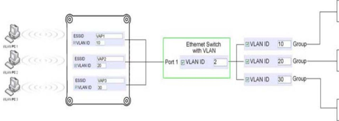
e.g. Virtual AP with SSID VAP1 has VLAN ID 10 and enabled WPA-PSK wireless security will be channeled to port 2 and 3 where the internet sharing router is connected.
