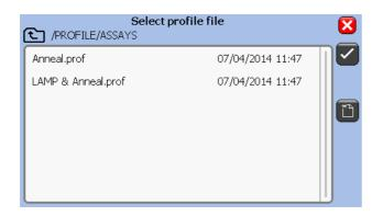
To create a new profile, press the 'Other...' button on the main screen. This allows access to any predefined profiles or creation of a new one. Cancel to return to the main menu.
