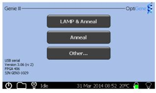
Up to four saved profiles can be shown on the main screen to allow quick starting of an assay. The four profiles are selected from the 'Buttons' page in the Toolbox.
