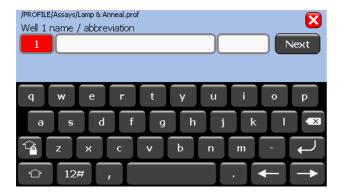
To change a well name, press on the text box and type a name and abbreviation if desired.
