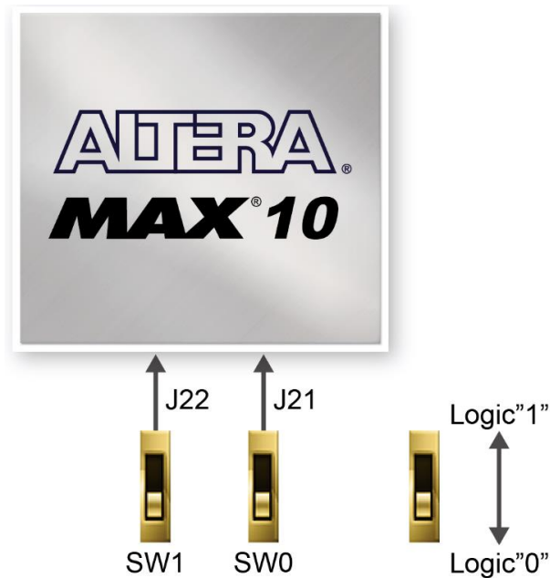
Figure 3-14 Connections between the slide switches and the MAX 10 FPGA
