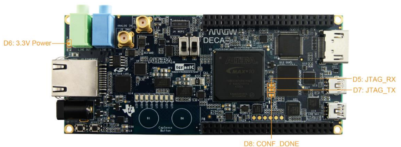
Figure 3-9 LED Indicators on DECA
