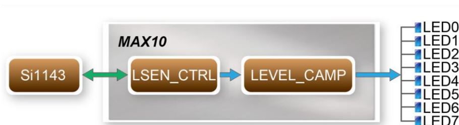
Figure 5-8 Block diagram of the Gesture Light Sensor
